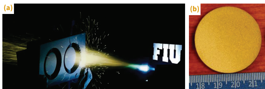
Fig. 1 — (a) Coating deposition using atmospheric plasma spraying at PFL, FIU. (b) Ti-hBN coating on a Ti6Al4V substrate.
